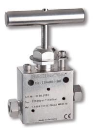
**MAXIMATOR** Sour Gas valves are designed for oil and gas service where  $H_2S$  is present. All valve bodies are made from annealed 316 stainless steel, with K-Monel stems in compliance with NACE MR0175. These needle valves with metal to metal seats have a high level of safety and reliability under harsh operating conditions. These valves may be used both with gases and liquids.
