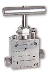
**MAXIMATOR** Sour Gas valves are designed for oil and gas service where  $H_2S$  is present. All valve bodies are made from annealed 316 stainless steel, with K-Monel stems in compliance with NACE MR0175. These needle valves with metal to metal seats have a high level of safety and reliability under harsh operating conditions. These valves may be used both with gases and liquids.
