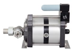
NOTE: L500 pumps have polyurethane seals and Buna-N O-rings and are available side inlet only. These pumps have UHMWPE seals and Buna-N O-rings. Maximum allowable oil/water temperature is 140°F. Air section temperature rating: 0°F to 140°F. 2Viton is a registered trademark of E.I. DuPont de Nemours & Co., Inc.
